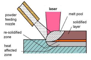
Fig. 3: Schematic of direct metal deposition.
