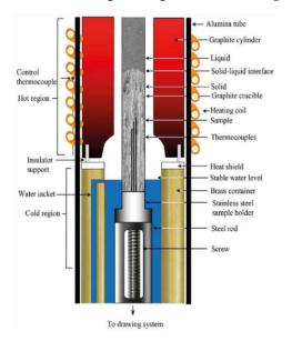
Fig. 1: Bridgman furnace scheme (Douglas, 2020).
