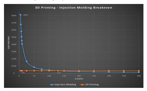
Fig. 2: Cost analysis of 3D printing vs injection moulding.
